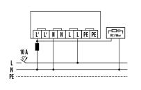
$Standard\ operation\ with\ optional\ parallel\ wiring\ of\ max.\ six\ motion\ detectors.$
